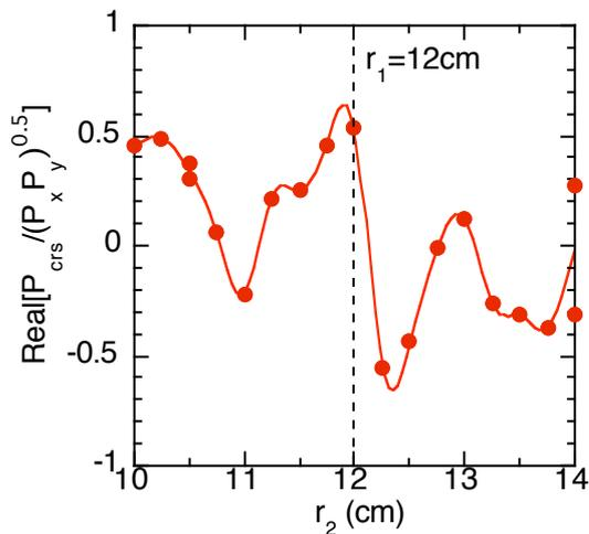
Figure 2. Phase difference of zonal flow in radial direction. The plotted points are the real part of the normalized cross power spectrum ( $\gamma \cos \theta$ ) between electric fields from the two HIBPs. In the measurements, the observation point of an HIBP is radially varied with the other fixed
