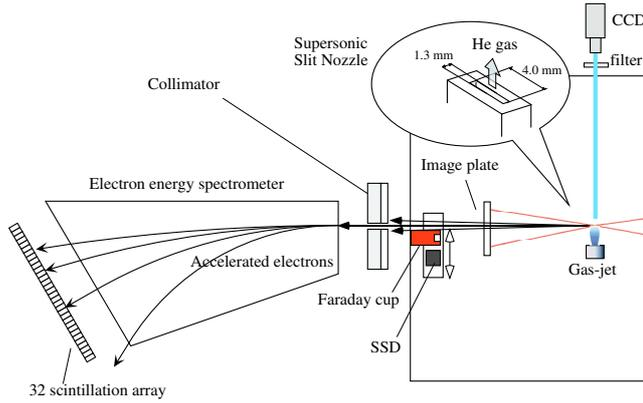
FIG. 1: A schematic of the experimental setup.
