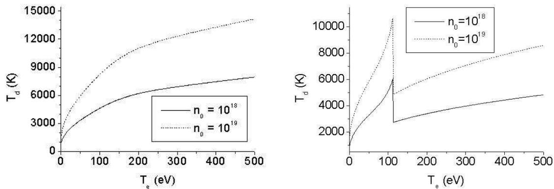
Figure 1. Steady state temperatures with  $T_i = T_e$  for a graphite dust grain (left), and a tungsten dust grain (right) for typical densities in  $\text{m}^{-3}$ .
