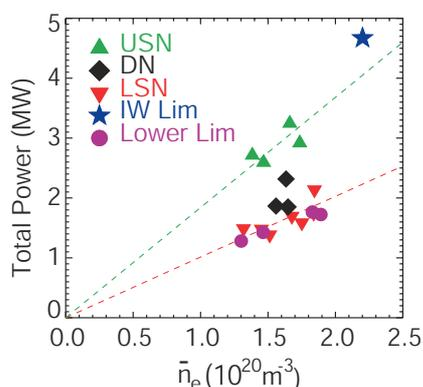
Figure 1. L-H threshold power vs  $\bar{n}_e$  for a set of 5.4 T, 0.8 MA discharges with different configurations.
