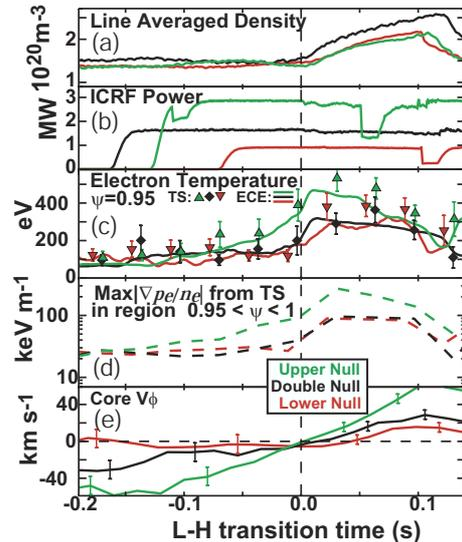
Figure 4: Comparison of rotation and edge parameters at L-H threshold in LSN, DN and USN configurations.
