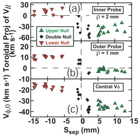
Figure 3: Variation with  $S_{sep}$  of toroidal projection of  $V_{||}$  at a) inner SOL, b) outer SOL and c) plasma center, for ohmic plasmas.
