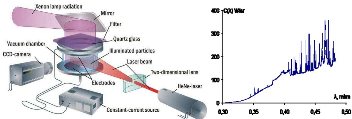
FIGURE 1. (a) Experimental setup; (b) Sunlight simulator emission spectrum.
