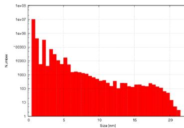
Figure 4: Distribution of nuclei on sizes obtained with the Frenkel-Raizer model for the  $125 \text{ J/cm}^2$  laser fluence at a gold target. The corresponding experimental data are presented in Fig. 2.
