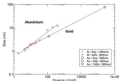
Figure 5: Size of nanoparticles on the laser fluence in aluminium and gold targets, for various laser wavelength, pulse duration.
