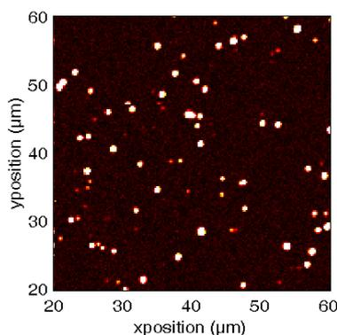
Figure 2: Substrate impacted by gold nano-particles. The incident laser fluence on the gold target is  $125 \text{ J/cm}^2$  and the substrate is located at 5 mm from the target. Image is obtained with a photothermal detection microscope.
