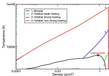
Figure 1: Temperature versus density thermodynamic diagram for aluminium. The binodal (1) limits the liquid-gas mixture domain from a gas (on the left from the critical point ) or from a liquid (on the right from the critical point). Curve 2 presents adiabatic expansion with droplets creation after a weak heating. Curve 3 presents adiabatic expansion with a partial recondensation after a strong heating. Curve 4 presents an adiabatic expansion with transition into the gas phase.
