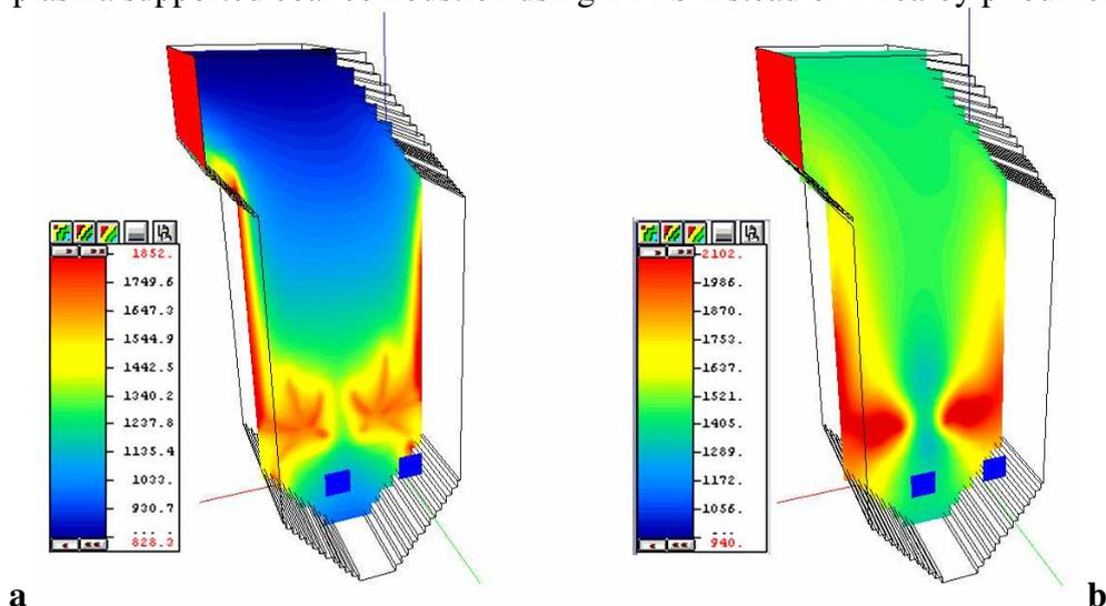
Fig. 3. Temperature fields along the furnace. (a) is conventional coal combustion, (b) is plasma supported coal combustion using 2 PFS instead of 2 nearby pf burners.
