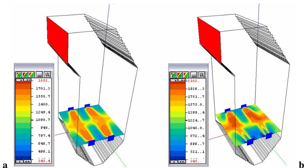
Fig. 2. Temperature fields on the level of the burners. (a) is conventional coal combustion, (b) is plasma supported coal combustion using 2 PFS instead of 2 nearby pf burners.
