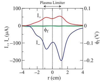
Figure 3: Radial profiles of the plasma with Ni grid.
