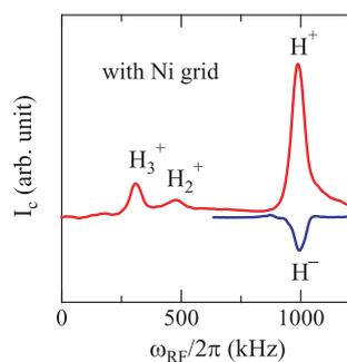
Figure 4: Mass spectra of the omegatron with Ni grid.
