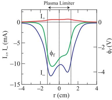
Figure 2: Radial profiles of the plasma without grid.
