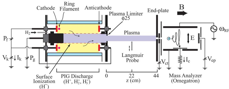
Figure 1: Schematic diagram of experimental setup.
