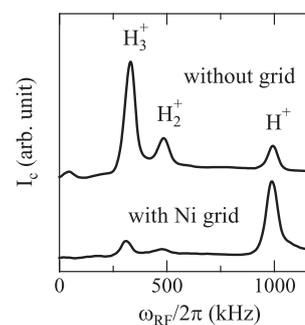
Figure 5: Mass spectra in the case of without and with Ni grid.
