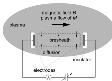
Figure 1: Schematic drawing of face-to-face double probe (FDP) and its measurement circuit.
