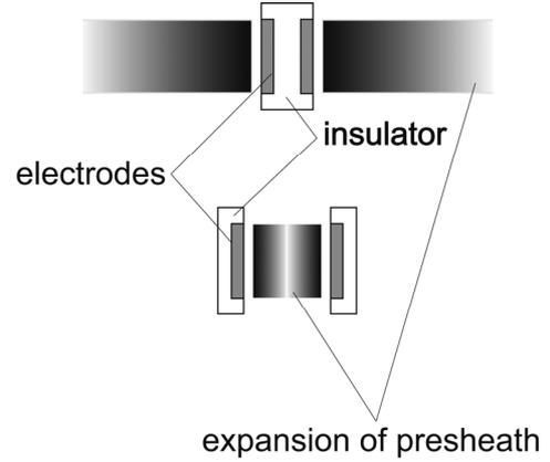
Figure 2: Difference in an expansion of presheath (gradation from black to white) between CMP (top) and FDP
