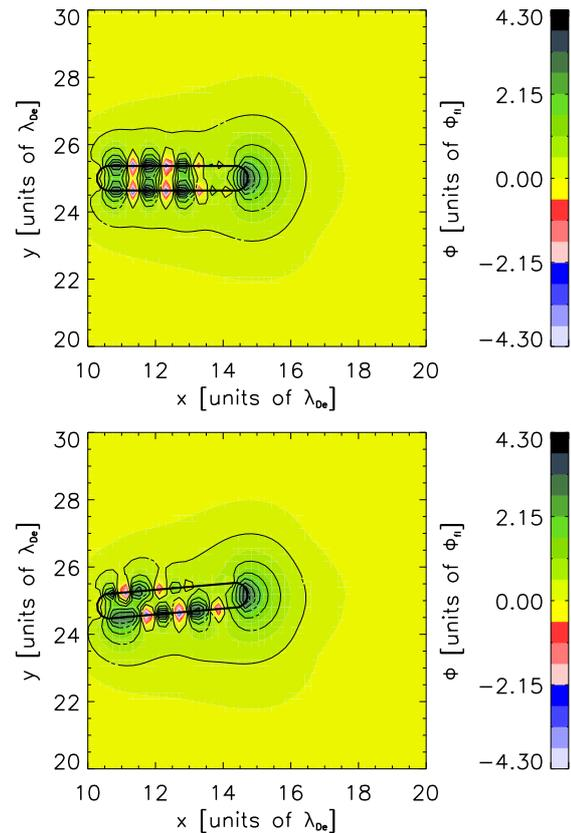
Figure 2: Potential variation for an insulating dust with the shape given by Fig. 1c) and the inclination angle  $\alpha = 0^\circ$  (top) and  $\alpha = 5^\circ$  (bottom) in a plasma with ion drift velocity  $v_d = 2.0 C_s$ . Potential is normalized with the floating potential  $\Phi_{fl} < 0$  consistent with our previous results [1]. The ion drift is in the positive  $x$ -direction.
