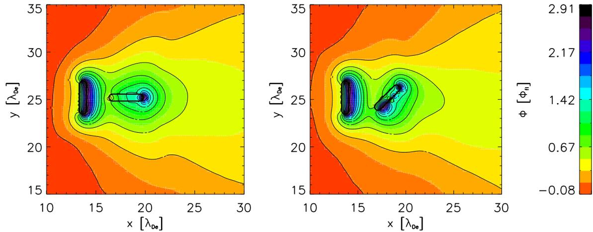
Figure 4: Potential variation for a plasma with ion drift velocity  $v_d = 2.0 C_s$  around two insulating rods with shapes given by Fig. 1b). Inclination angles are  $\alpha = 90^\circ$  for the rod facing the flow, and  $\alpha = 0^\circ$  and  $\alpha = 45^\circ$  for the rod in the wake. Potentials are normalized as in Fig. 2, but the color scale is different. The ion drift is in the positive  $x$ -direction.
