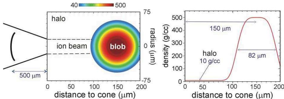
**Figure 1.** Density iso-contours and central cut of the compressed fuel used in our simulations. We assume that the ion source is located in the hollow cone depicted at the left, 500  $\mu\text{m}$  from the surface of the simulation box.
