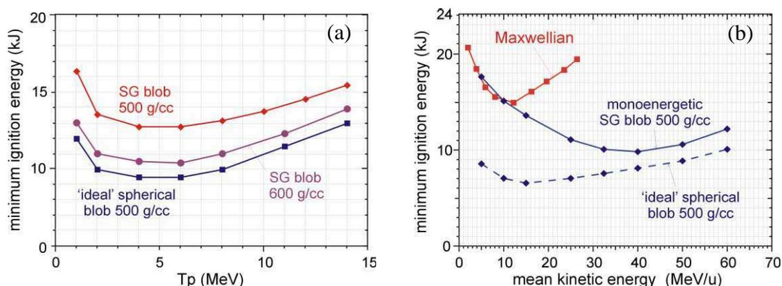
**Figure 3.** Ignition energies of the target shown in Fig. 1 heated by (a) proton and (b) carbon beams as a function of the temperature and specific beam kinetic energy, respectively. SG stands for supergaussian density profile with the peak density shown and ‘ideal’ for isochoric plasma.
