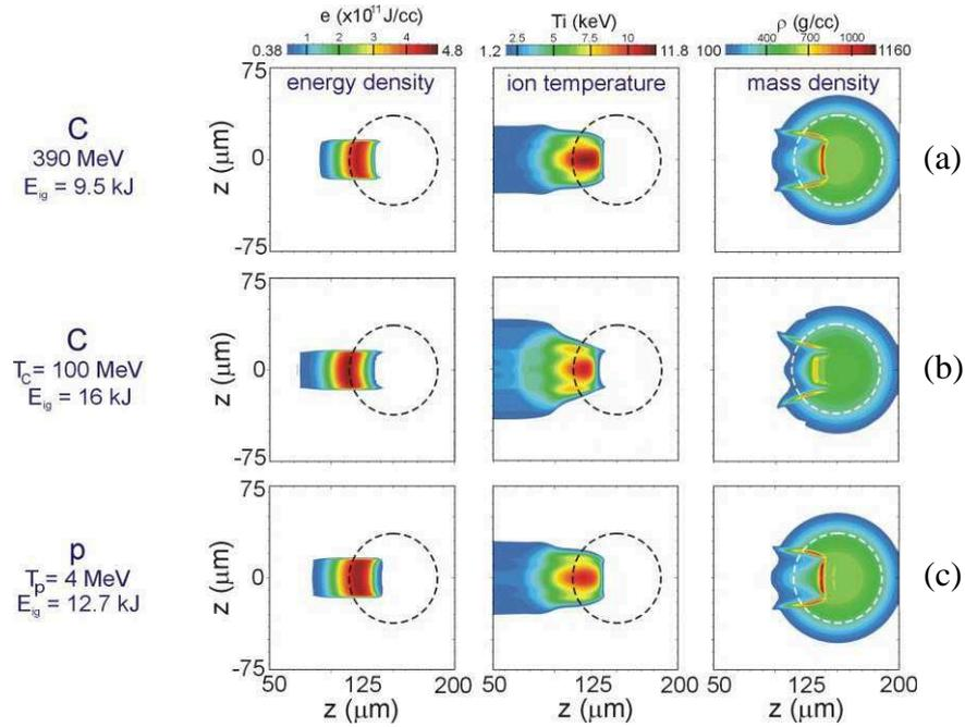
**Figure 2.** Energy density deposited by (a) a carbon beam with a mean kinetic energy of 32 MeV/nucleon and 10% of energy spread, the ignition energy is  $E_{ig} = 9.5$  kJ (b) carbon beam with a Maxwellian energy distribution and temperature  $T_C = 100$  MeV,  $E_{ig} = 16$  kJ, and (c) proton beam with a Maxwellian energy distribution and  $T_p = 4$  MeV,  $E_{ig} = 12.7$  kJ. DT density is higher than  $250$  g/cm<sup>3</sup> within the encircled areas.
