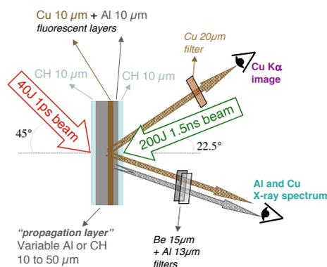
Figure 1: In-principle scheme of the experimental set-up and of the used targets.
