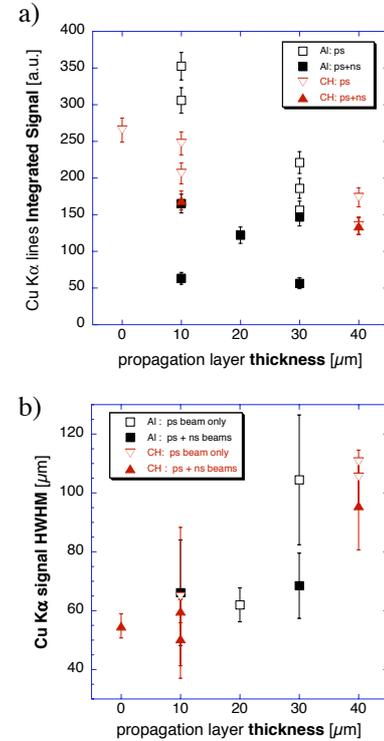
Figure 4: **a)** Cu  $K\alpha$  spectral lines integrated emission and **b)** Cu  $K\alpha$  spot radius (HWHM) as a function of the propagation layer thickness.
