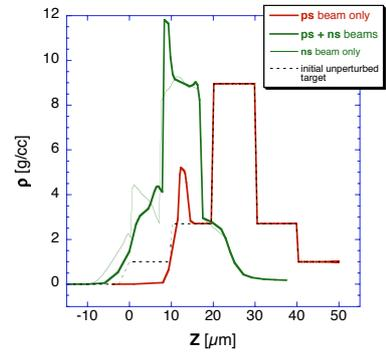
Figure 2: CHIC hydrodynamic calculation: Density profiles for a  $10\mu\text{m}$  Al propagation layer target at the intense ps pulse arrival moment.
