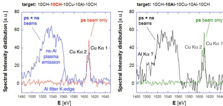
Figure 3: Typical X-ray spectra: solid vs. shock compressed targets for dielectric (left) and conductor (right) propagation layers.
