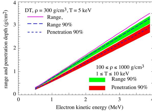
Figure 2: From 3D Monte Carlo simulations: electron range and penetration depth vs initial electron energy.
