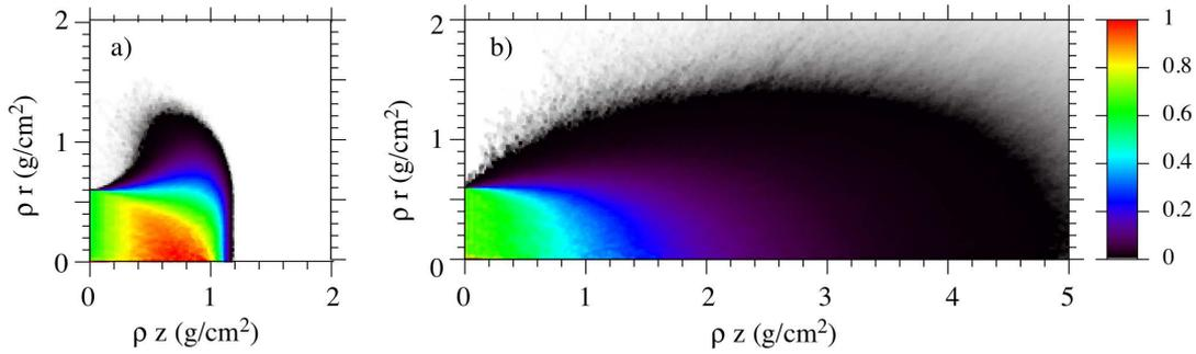
Figure 3: Specific power deposited by a) a beam of 1.5 MeV electrons and b) a beam with exponential energy distribution (with average energy of 1.5 MeV). In both cases a parallel beam impinges from the left h.s. on a DT plasma slab, with  $\rho = 300 \text{ g/cm}^3$  and  $T = 5 \text{ keV}$ .
