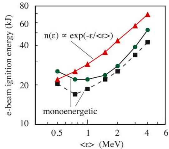
Figure 4: Minimum electron beam energy required for the ignition of a uniform DT sphere, initially at rest, and with mass density  $\rho = 300 \text{ g/cm}^3$ . The dashed curve refers to simulations neglecting scattering.
