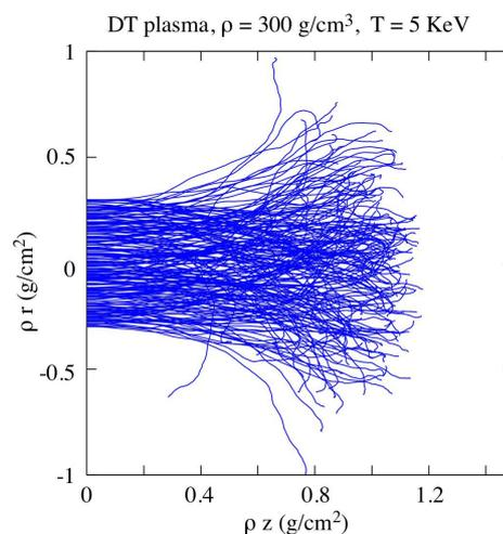
Figure 1: Trajectories of a beam of 1.5 MeV electrons incident on a plasma slab
