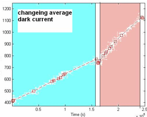
Fig.8. Change of average dark current at 20ms exp. time
