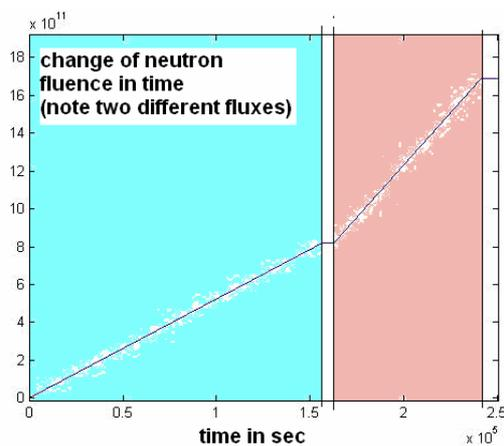
Fig.6 Change of fluence during neutron irradiation
