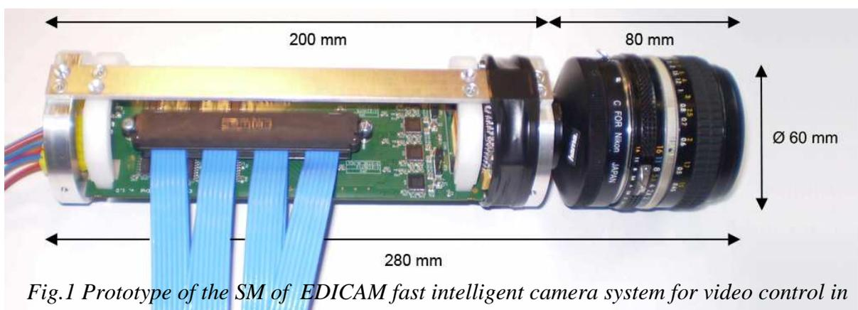
*Fig.1 Prototype of the SM of EDICAM fast intelligent camera system for video control in fusion devices prepared for test*
