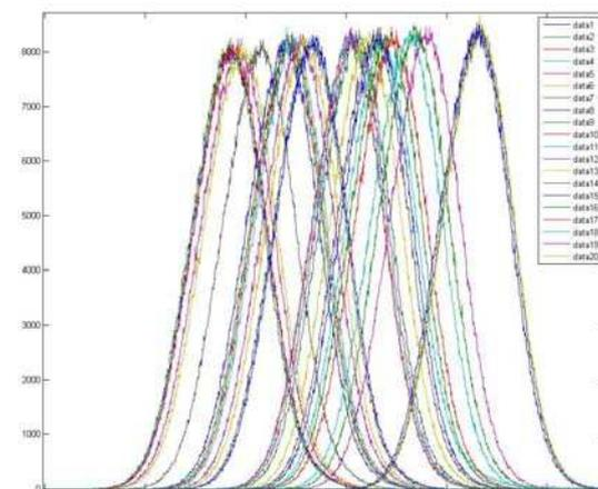
Fig 7. Shift of distribution function of dark current on picture taken with 2 ms exposure time
