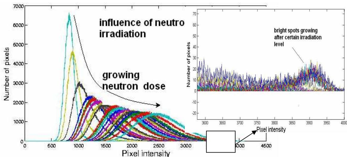
*Fig.10. Shift of distribution (200msec exp.time), the originally high kurtosis falls to normal*
