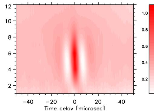
Figure 6. 2D correlation function in an ohmic discharge. The reference channel is inside the LCFS. The colour scale corresponds to the relative fluctuation amplitude (%).
