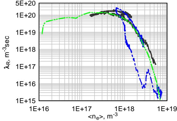
Figure 3. Trends in runaway electron generation:  $\lambda_R$  calculated vs. plasma density for several shots in ISTTOK
