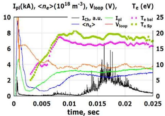
Figure 2. Typical evolution of the main plasma parameters including the evolution of calculated electron temperature and the signal from the detector of Cherenkov radiation.
