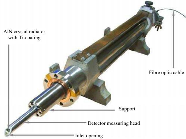
Figure 1. View of the detector used for the measurements of Cherenkov emission in ISTTOK.
