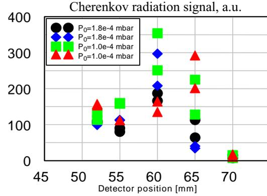
Figure 4. Spatial characteristics of the Cherenkov radiation obtained in the different series of the ISTTOK discharges.
