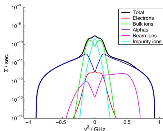
Figure 1: Scattering function for location in the NBI beam path, resolving near parallel velocities; scattering parameters:  $R = 5.9m$ ,  $Z = 0.58m$ ,  $\phi = 6^\circ$ ,  $\theta = 22^\circ$ ,  $\psi = 176^\circ$
