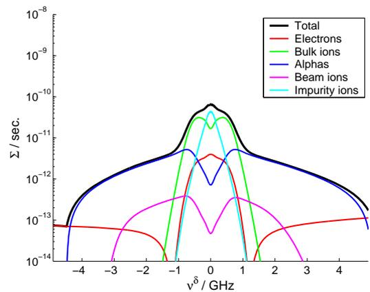
Figure 2: Scattering function for location in the NBI beam path, resolving near perpendicular velocities; scattering parameters:  $R = 6.0m$ ,  $Z = 0.62m$ ,  $\phi = 101^\circ$ ,  $\theta = 163^\circ$ ,  $\psi = 7^\circ$
