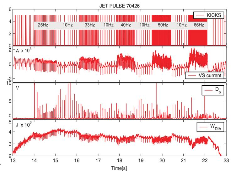
Fig 4: Pulse 70426: rapid variation of kick frequency corresponds immediate plasma change in frequency. This proves that the plasma has no memory of the kick. Note how the VS current grows with the increase of the frequency.
