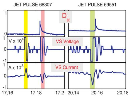
Fig 1: Voltage response to a natural ELM (pink bar), a positive kick (yellow bar), and a negative kick (green bar). The kick direction (positive/negative) is determined by the initial sign of the voltage. The following counter-kick is the VS trying to recover plasma vertical control. Note that in the natural ELM the VS applies a positive voltage briefly. This is caused by a measurement problem.
