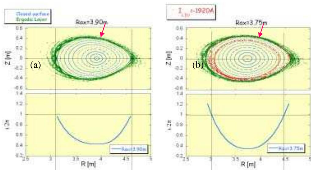
Fig. 1 Cross section of closed magnetic surface and ergodic layer at the toroidal section locating the diagnostics (upper) and radial profile of rotational transform (bottom). The magnetic configuration of magnetic axis position ( $R_{ax}$ ) is (a) 3.90m and (b) 3.75m. In the case of  $R_{ax}=3.75m$ , expanded  $m/n=1/1$  magnetic island is also plotted (red dots).
