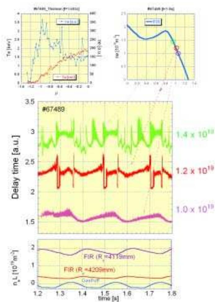
Fig. 2 (a) Radial profile of electron temperature and density measured by Thomson scattering. (b) Radial profile of electron density measured by FIR interferometer. (c) Temporal behaviour of ToF of reflected pulses from corresponding cut-off layer. (d) Temporal behaviour of line integrated electron density and modulated gas puff signal.
