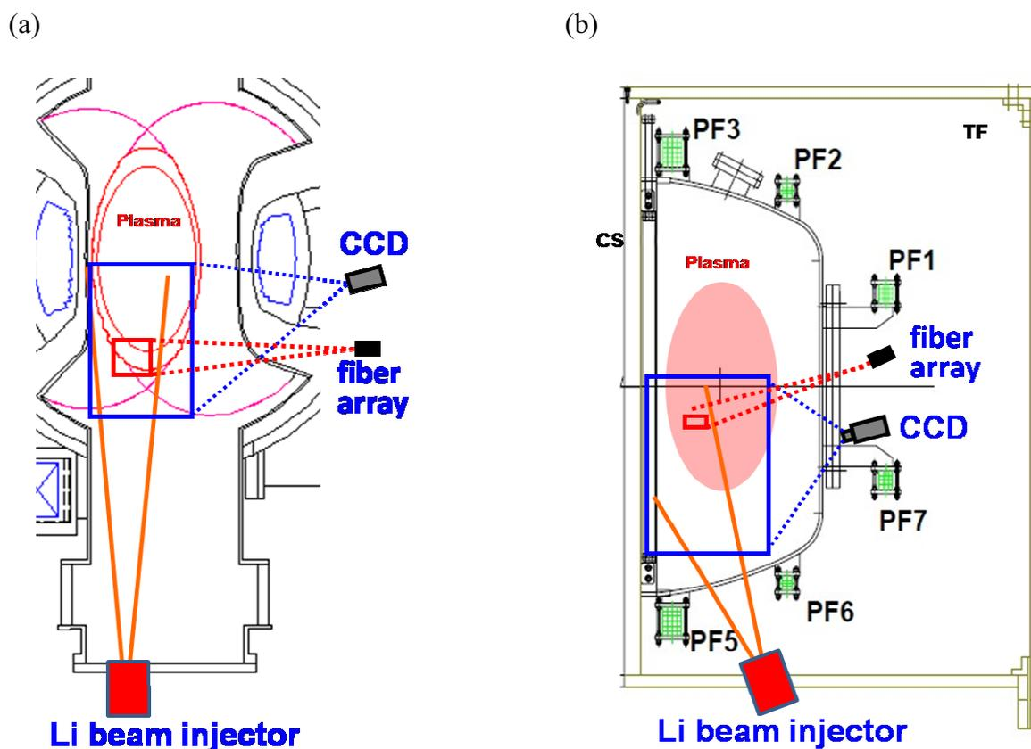
Fig. 1. Schematics of 2D-LiBP for (a) LHD and (b) CPD.
