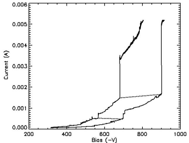
**Figure 4:** Jumps in the emission current as the emitter bias is increased. Left curve is at  $B = 0.01T$ , right curve at  $B=0.014T$ .
