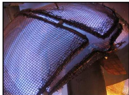
**Figure 2:** Copper mesh conforming to the magnetic surfaces installed in CNT.
