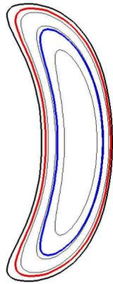
**Figure 3:** Plasma cross section at  $\varphi = 0^\circ$  and surfaces outside which there are unconfined orbits in the case of: **Blue** potential with no conforming boundary, **Red**: potential constant on surfaces. Also plotted are the magnetic surfaces  $\psi=0.25,0.5,0.75$  and 1.
