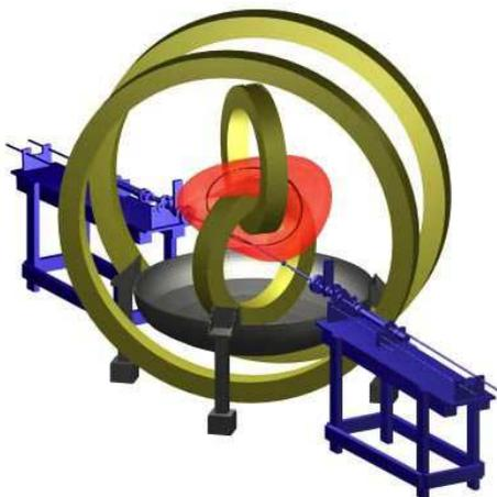
**Figure 1:** Cutaway view of the CNT device with the four coils, the plasma volume and the probes.
