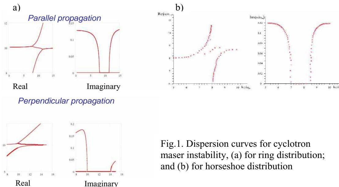
Fig.1. Dispersion curves for cyclotron maser instability, (a) for ring distribution; and (b) for horseshoe distribution
