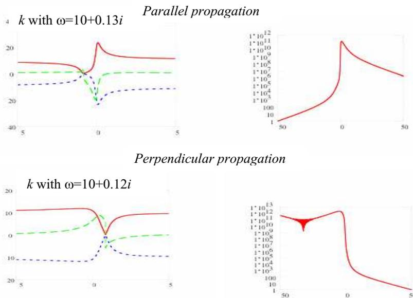
Fig.3. Dispersion curves (a,c) and field amplitude (b,d) for smooth gradient of B; red and blue are real parts of positive and negative square roots and green is imaginary part corresponding to red line.
