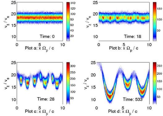
Figure 1: The electron phase space density in units of simulation electrons: (a) Initial distribution. (b) The  $B_y$  grows but not yet  $E_x$ . (c) The  $E_x$  component grows too. (d)  $B_y$  and  $E_x$  are in a steady state.
