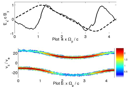
Figure 2: The fields at  $t\Omega_p = 533$  are shown in (a), where  $B_y$  is dashed and normalized to 275 V/m and  $E_x$  (solid line) is normalized to 50.5 V/m. (b) is the electron phase space distribution.
