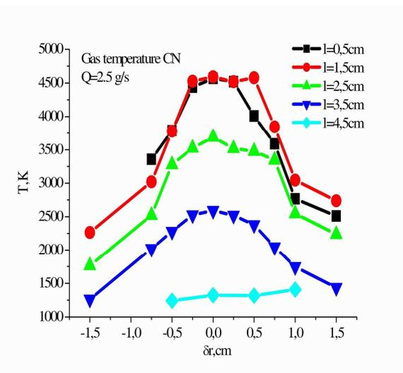
**Figure 6.** Cross-profile of gas temperature at gas flow  $Q=2.5$  g/s on different distance  $l$  from nozzle section obtained with comparison modeling with experimental spectrums.
