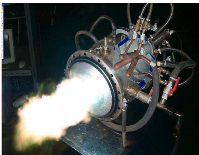
**Figure 2.** Photo and principal scheme of multi-phase powerful alternating current plasma generator.
