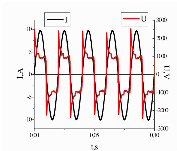
**Figure 3.** Time dependences of current I and arc- voltage drop U.
