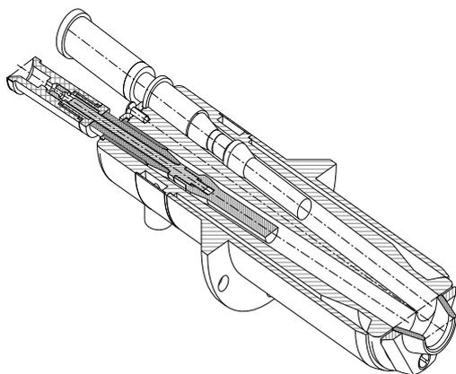
**Figure 1.** Principal scheme of single-phase alternating current plasma generator
