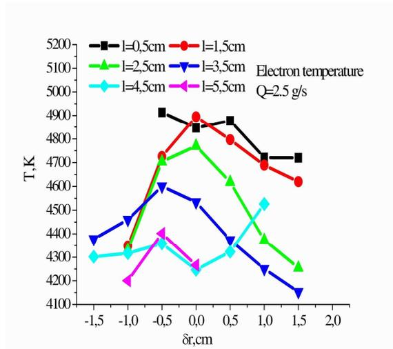
**Figure 5.** Cross-profile of electron temperature at gas flow  $Q=2.5$  g/s on different distance  $l$  from nozzle section
