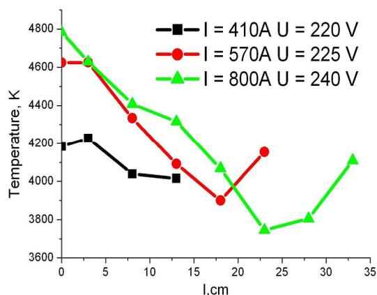
**Figure 6.** Inline-profile of temperature in the centre of the multi-phase plasma generator's torch at gas flow  $Q=30$  g/s on different distance  $l$  from nozzle section.  $I$ ,  $U$  - active value of the arc's current and voltage correspondingly.
