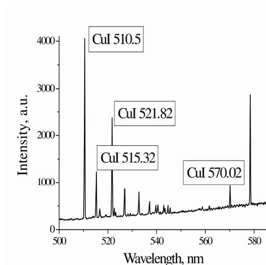
**Figure 4.** Emission spectrum of copper atoms.
