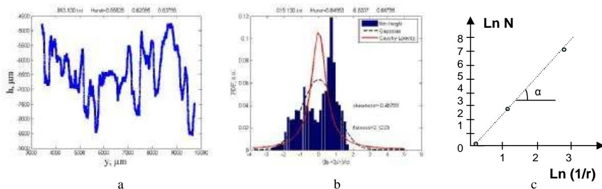
Fig.3 –data from profiler (a), functions of distribution increments of heights  $\Delta h$  (b). Identification of self-similarity (c)
