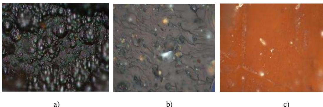
Fig.2 – Photo (100x 70  $\mu\text{m}$ ) by Olympus GX-51, a - films near limiter , b - 90 from limiter, c - 180 from limiter.
