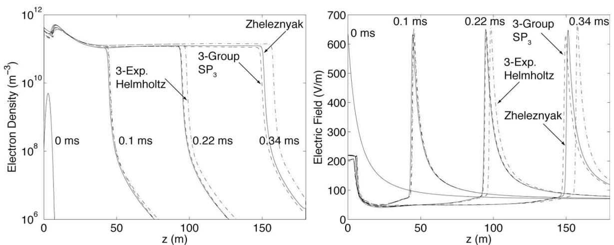
**FIGURE 2** Electron density (left) and electric field (right) profiles along the symmetry axis of the computational domain for the moments of time from  $t=0$  to  $t=0.34$  ms calculated using different photoionization models.
