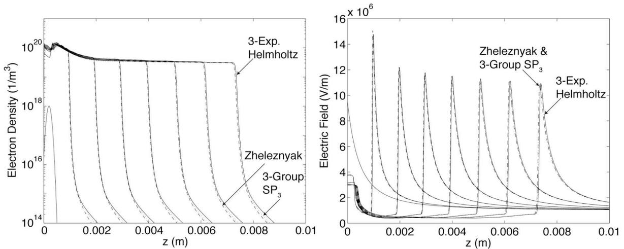
**FIGURE 1.** Electron density (left) and electric field (right) profiles along the symmetry axis of the domain for the moments of time from  $t=0$  to  $t=17.5$  ns, with a timestep of 2.5 ns calculated using different photoionization models.
