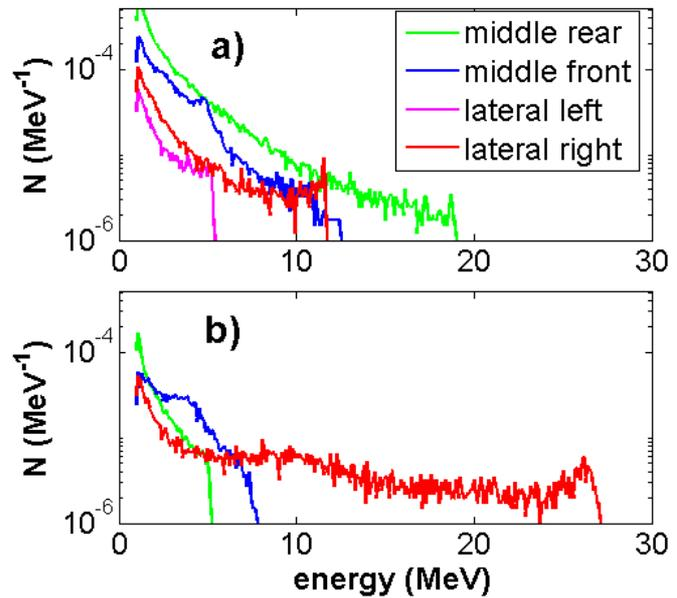
Figure 1: Proton energy spectra for angles of incidence a)  $30^\circ$ , b)  $75^\circ$ . Only protons with energy higher than 1 MeV are taken into account. In the case b), lateral proton emission from the left side is very weak and the cutoff energy of protons is about 0.7 MeV there. Lateral right side is in the direction of the laser wave vector projection onto the front target surface.
