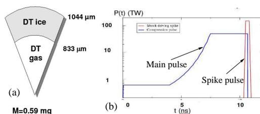
Figure 1: (a) All DT target baseline. (b) Main pulse shape to obtain a low adiabat shell during the compression phase and spike pulse required for shock ignition, about  $\sim 80$  kJ during  $\sim 400$  ps (150-200 TW).
