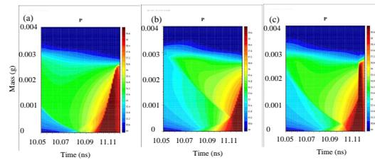
Figure 2: Pressure vs time in mass coordinate around the shell stagnation. (a) the spike is launched too early (b) too late and (c) on time.
