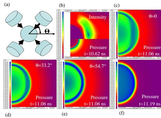
Figure 4: (a) set-up of the ignitor beams with incident angle  $\theta$ . (b) Laser absorbed power and pressure during the spike irradiation for  $\theta = 0$ . (c) 440 ps later: pressure during the shock-ignitor propagation inside the hot spot (c) for  $\theta = 0$ , (d) for  $\theta = 33.2^\circ$  (e) for  $\theta = 54.7^\circ$ . (f) Pressure becomes isotropic for the three angles 130 ps latter.
