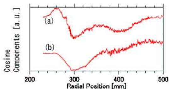
Fig. 6 Waveforms of cosine components of (a) toroidal, extraordinary and (b) vertical, ordinary wave.
