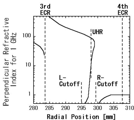
Fig. 3 Profile of perpendicular refractive index for 1.0 GHz injection.
