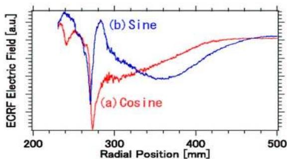
Fig 5 Radial profile of electrostatic ECRF electric field (a)Cosine and (b) Sine component.
