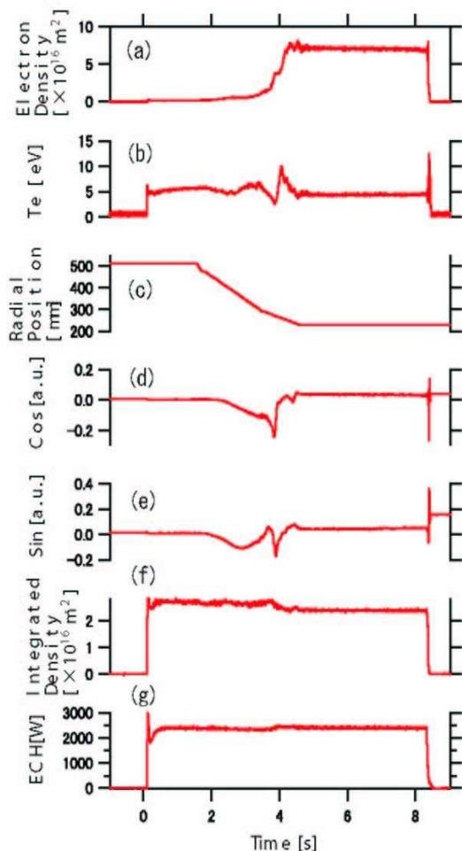
Fig. 4 Typical waveforms of (a) electron density, (b) electron temperature  $T_e$ , (c) radial position of antennas and Langmuir probe, (d), (e) Cosine and sine component of electrostatic ECRF electric field (f) line integrated density and (g) ECH power.
