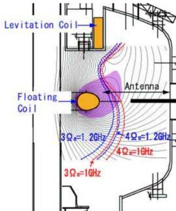
Fig. 1 Magnetic Configuration in the Mini-RT device.
