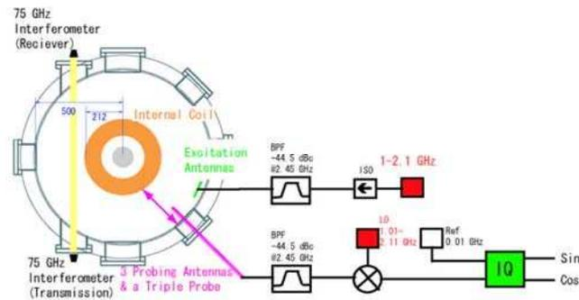
Fig. 2 Diagram of ECRF electric field measurements; we used two dipole antenna (element lengths are 40 mm) and a small monopole antenna (1 mm length).
