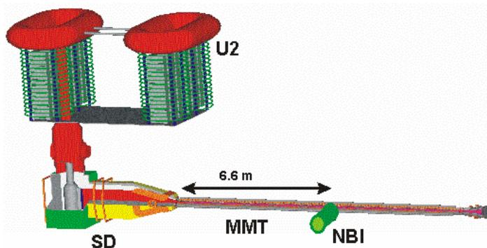
Fig.1. Layout of NBI system at GOL-3 facility; U2 - electron beam generator, SD - sheet electron beam diode, MMT - multimirror trap, NBI - neutral beam injector.
