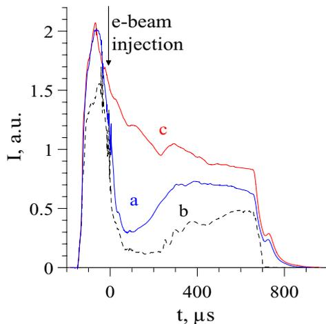
Fig. 4. Waveforms of the beam current at the beam dump: a, b – with plasma in two regimes similarly labeled in Fig. 2; c - vacuum only.
