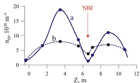
Fig. 2. Initial gas pressure distribution along the facility; a and b are two operation regimes studied in experiments.
