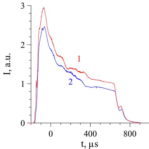
Fig. 3. Waveforms of the beam current at the beam dump: 1 – vacuum only, 2 – gas-filled chamber.
