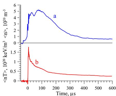
Fig. 6. Waveforms of plasma density (a) and diamagnetic pressure (b).
