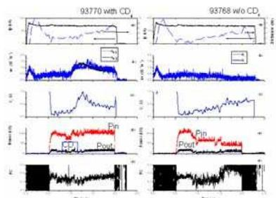
Fig. 3 Waveforms of with and w/o CD<sub>4</sub> puffing with varied distance in one discharge
