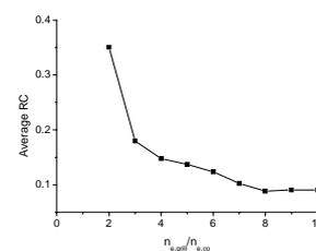
Fig. 5 Calculated reflection coefficient vs grill mouth density
