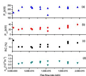
Fig. 4 Effect of gas flow rate on wave-plasma coupling
