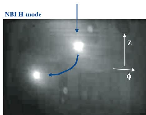
Fig. 4. A tangentially viewing fast camera image showing the light emitted by two dropper pellets. The top pellet has just started ablating in the scrape off layer. The lower pellet is an earlier pellet that has been swept toroidally while ablating by effects from the SOL plasma.
