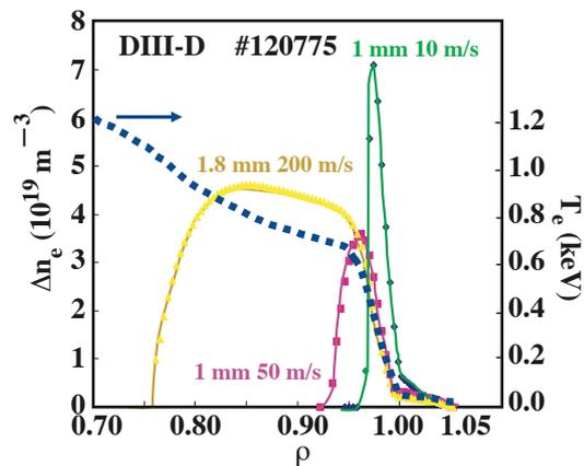
Fig. 3. Pellet mass deposition profiles calculated with the PELLET code for typical H-mode profiles. No mass drift is included in the deposition calculation.
