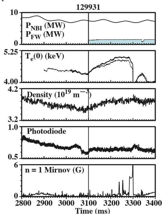
Fig. 2. The first 0.3 s of the FW pulse into an H-mode in which ELMs have been suppressed with RMP. The top trace shows the neutral beam and the total FW power, the second trace shows the central electron temperature from ECE (2 channels), the third trace, the line-averaged density, the fourth trace, an edge  $D_{\alpha}$  signal, and the bottom trace,  $n=1$  Mirnov signal.
