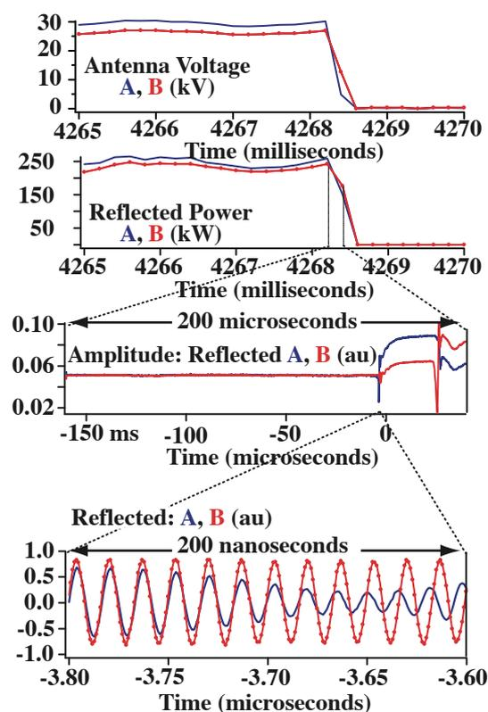
Fig. 3. Illustrating the first application of the ultra-high-speed data acquisition system to study an antenna arc into an H-mode plasma at 30 kV peak antenna voltage at the millisecond, microsecond, and nanosecond timescales. The arc begins on side “A” of the system a few microseconds before it is detected and the generator commanded to shut down.
