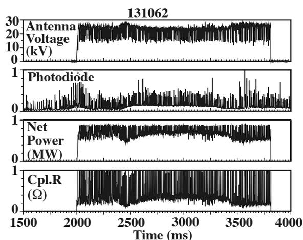
Fig. 1. Arc-free operation of the 285/300 antenna array at up to 28 kV peak in a vigorously ELMing H-mode. From top to bottom, time histories of peak antenna voltage, the  $D_{\alpha}$  light from the edge of the plasma, the net 60 MHz power level applied to the array and the coupling resistance per antenna element are shown.
