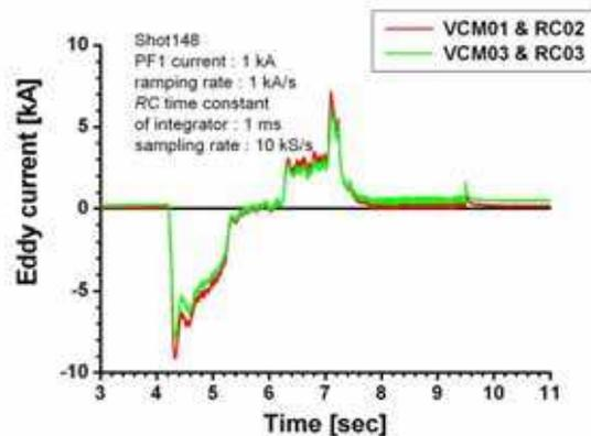
Figure 5. Eddy current evaluated from the VCM and RC signals in Fig. 3.
