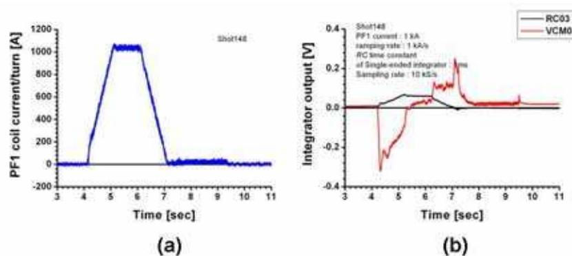
Figure 4. Performance test of the VCM and RC during the commission of the PF coil after the cool-down of the superconducting magnet: (a) the wave form of the PF1 coil current and (b) VCM and RC signals.
