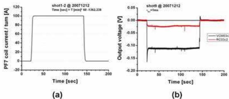
Figure 2. Poloidal flux measurement: (a) a typical waveform of a low pulse current applied to PF7 coil pair and (b) VCM and RC signals. Here, VCM03 and RC01 mean vessel current monitor and Rogowski coil, respectively.
