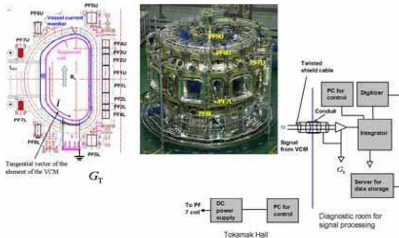
Figure 1. Experimental set-up for the flux measurement before the cool-down of the magnet coils.
