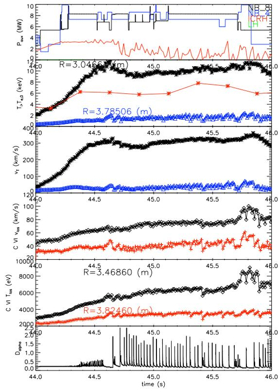
Figure 2: Data during JET pulse 72743, showing (a) the auxiliary power, (b) “core” CXRS measured  $T_i$  at two different radii and  $T_{e,0}$  from LIDAR (red), (c) toroidal rotation,  $v_\phi$ , (d) “edge” CXRS measured line-of-sight rotation at two radii from the  $C v_i$  line, (e) apparent temperature, and (f) a  $D_\alpha$  trace.
