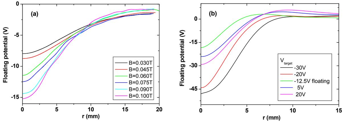
Fig. 3. Radial profile of the floating potential, having as parameter: (a) the magnetic field; (b) the target bias (at  $B = 0.4$  T).
