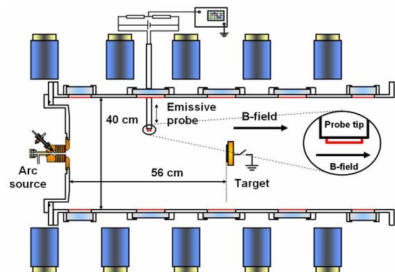
Fig. 1. Pilot-PSI experimental set-up
