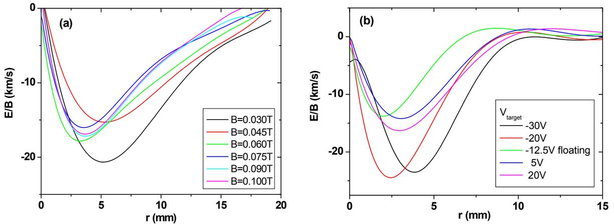
Fig. 4. Radial profile of  $E/B$  velocity having as parameter: (a) the magnetic field; (b) the target bias (at  $B = 0.4$  T).
