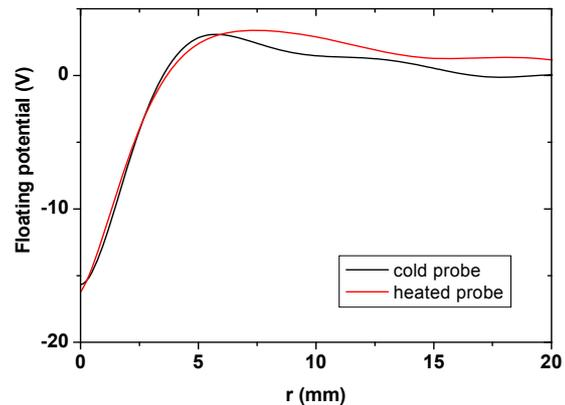
Fig. 2. Radial profile of the floating potential measured with both cold and emissive probes ( $I_d = 120 \text{ A}$ ,  $p = 1.6 \text{ Pa}$ ,  $B = 0.4 \text{ T}$ )
