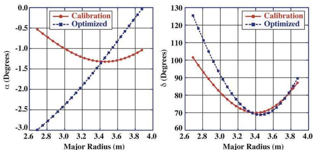
Fig 2. Comparison of laboratory measured calibration coefficients with those from a combined optimization of  $\alpha$  and  $\delta$  and a fixed value of  $a_{23}$ . The difference is within the experimental error in the measurement of the calibration coefficients.
