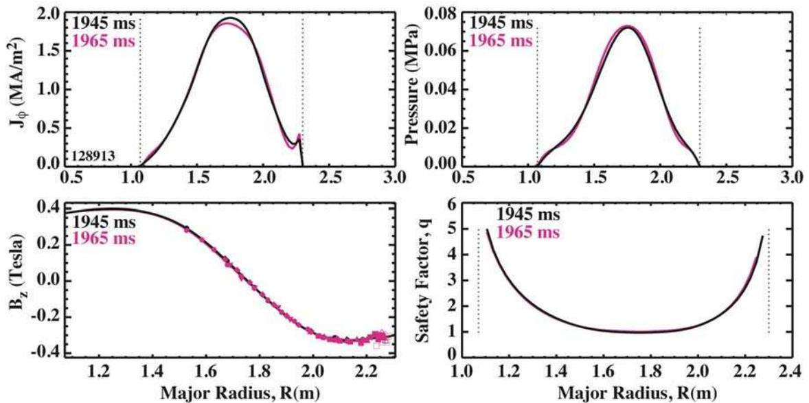
Fig 1. Profiles before and after a transition from a single MSE co-beam (black curves) to both a co- and counter MSE beam (magenta curves) based on a simplex optimized calibration. Symbols indicate locations of individual MSE channels.
