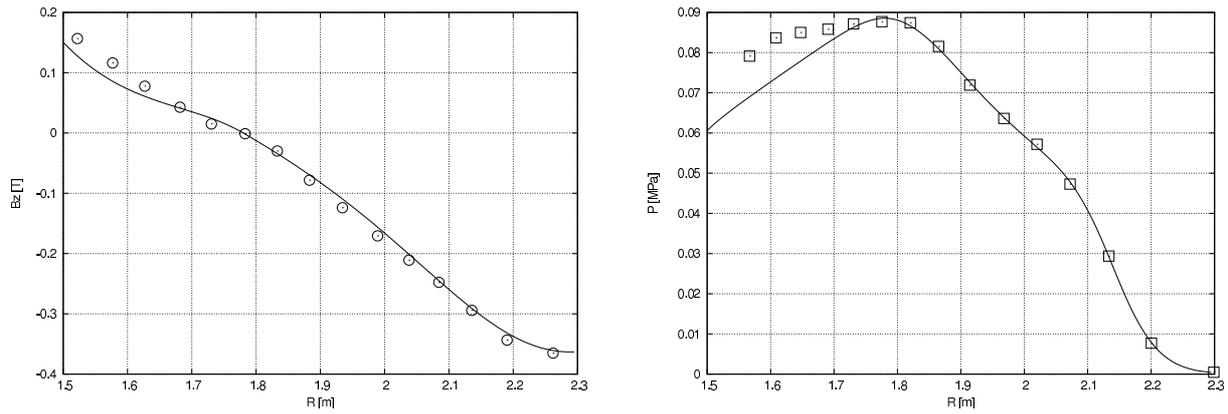
Figure 2: Measured vertical field  $B_z$  (open circles) and plasma pressure  $P$  (open squares) together with the corresponding reconstructed profiles (solid line).
