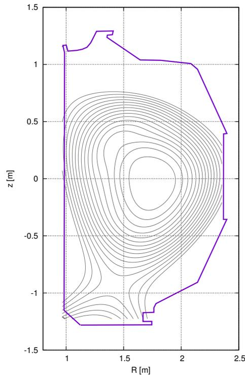
Figure 1: Surfaces of constant poloidal-field flux.
