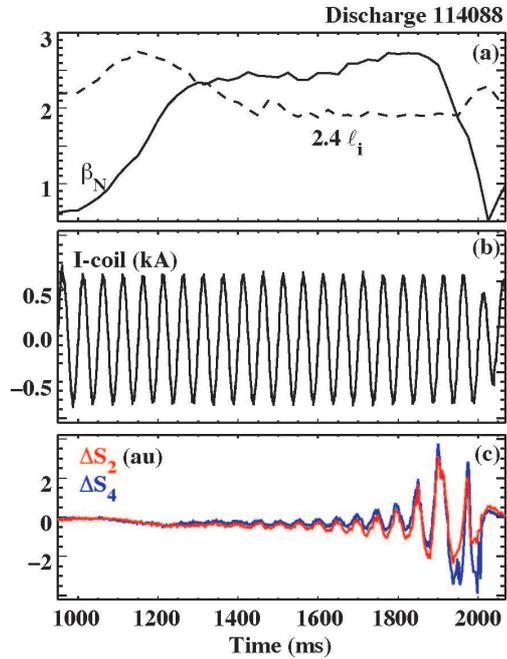
Figure 1: (a) With  $\beta_N$  above the no-wall limit, (b) the I-coil applies a rotating field at 20 Hz. (c) The RFA is observed on the  $\Delta S_i$ .
