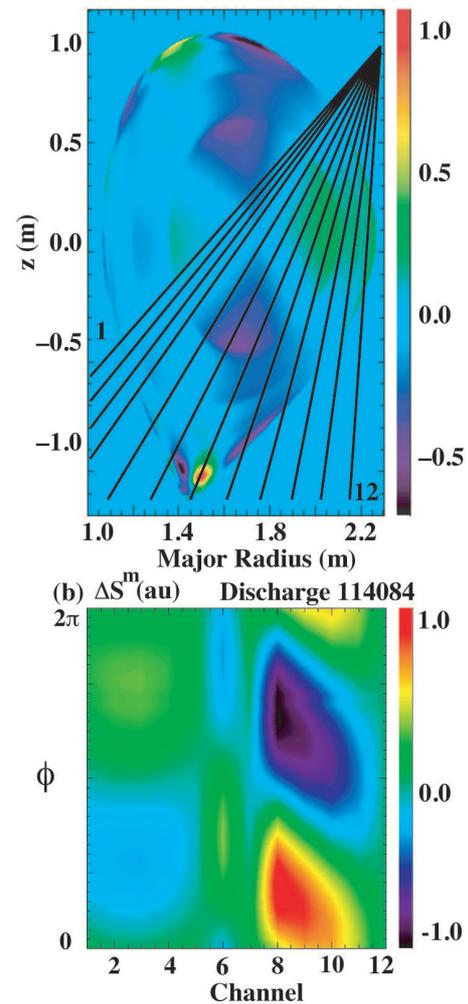
Figure 2: (a) Normalized  $\xi \cdot \nabla\psi$  from GATO with centerlines of SXR viewing chords. (b) Modeled  $\Delta S^m$  as a function of toroidal angle.
