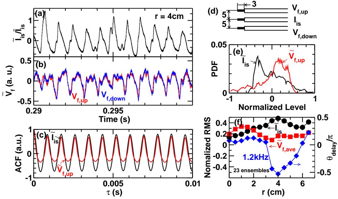
Figure 1: Typical time evolutions of (a) the  $\tilde{I}_{is}$  and (b) the  $\tilde{V}_{f,up/down}$  and (c) their auto-correlation functions. (d): The schematic view of 2-D movable probe tips. (e): Probability density functions corresponding to time series of (a) and (b). (f): Radial profile of normalized amplitude of the  $\tilde{I}_{is}$  and the  $\tilde{V}_{f,ave}$  and phase delay between  $\tilde{I}_{is}$  and the  $\tilde{V}_{f,ave}$  at 1.2kHz.
