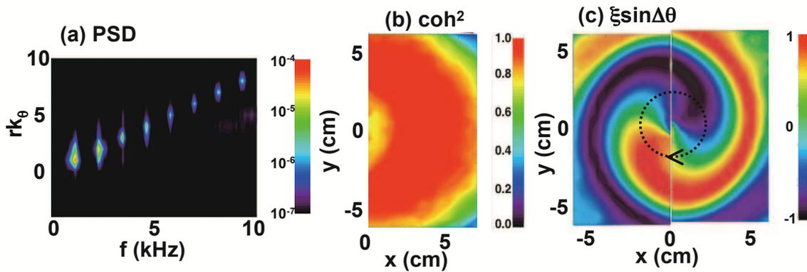
Figure 2: (a): Power spectrum in frequency-wave number space at  $r = 4$  cm. Two dimensional structures of (b) squared coherence and (c) imaginary part of cross-spectrum for the coherent mode at 1.2 kHz. The arrow denote the direction of propagation (the electron diamagnetic drift direction).
