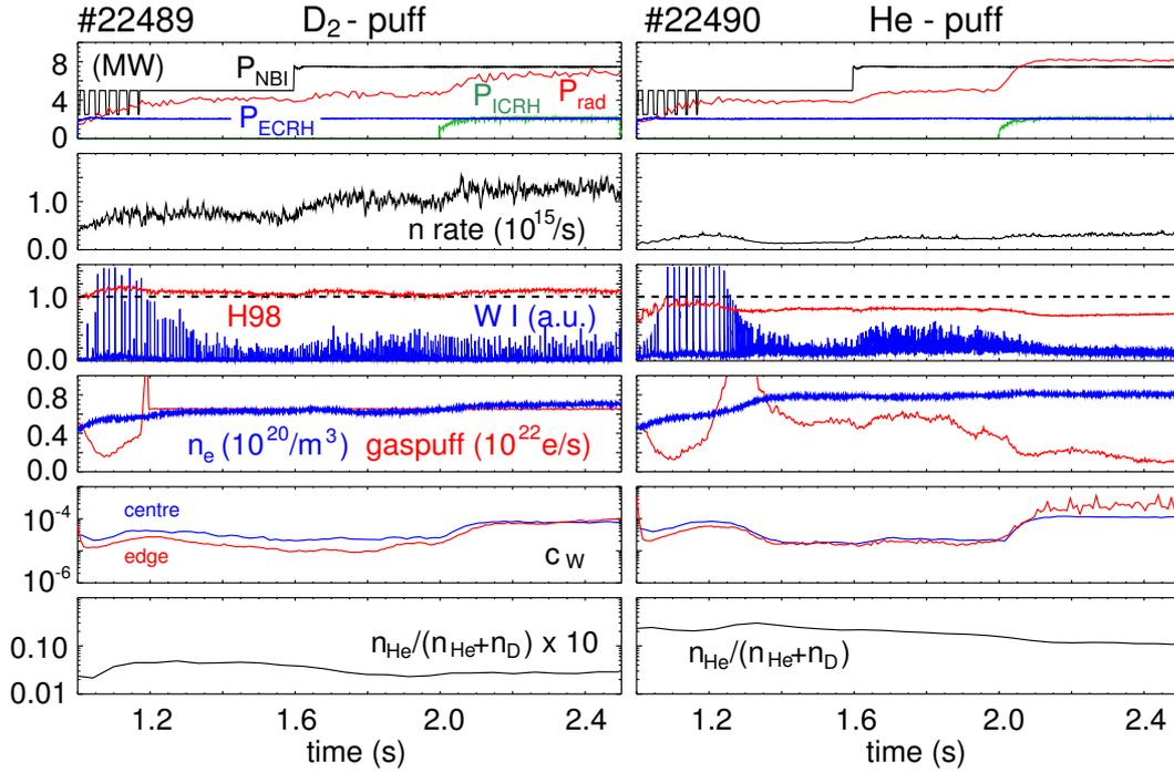
Figure 2: Comparison of discharges with D<sub>2</sub> (#22489, left-hand side) and He puffs (#22490, right-hand side) and otherwise similar technical parameters. The parameters from top to bottom are: Auxiliary heating power (NBI, ECRH, ICRH) and radiated power; neutron rate; ITER98 H-factor and W I divertor radiation; line averaged density and gas puff rate (electrons/s); central and edge W concentration; He concentration.
