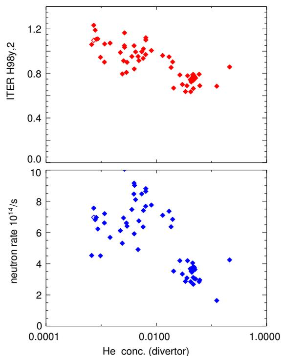
Figure 1: ITER H98y,2 factor and neutron rate versus He concentrations in the divertor.
