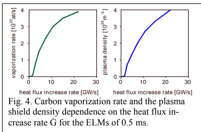
Fig. 4. Carbon vaporization rate and the plasma shield density dependence on the heat flux increase rate  $\dot{G}$  for the ELMs of 0.5 ms.
