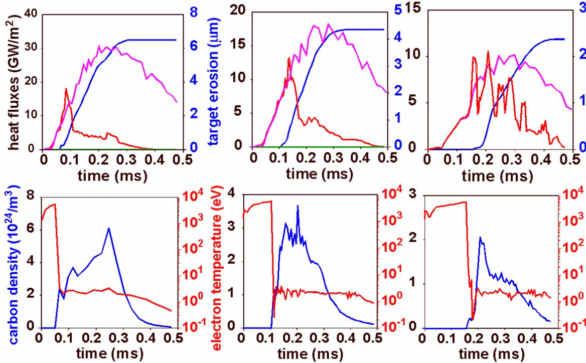
Fig. 3. Time dependences for the heat flux to the divertor armour without shielding, for the shielded heat flux and for the erosion, shown in the upper panel. Corresponding time dependences for carbon plasma density and temperature close to the armour are in the lower panel. The three columns correspond for the heat flux increase rate  $\dot{G}=220 \text{ GW/m}^2/\text{ms}$ ,  $\dot{G}=106 \text{ GW/m}^2/\text{ms}$  and  $\dot{G}=52 \text{ GW/m}^2/\text{ms}$ .
