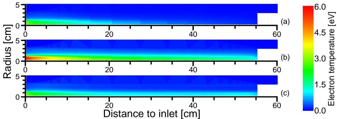
Figure 2:  $T_e$ -profile of the three simulations as given in Table 1. In (a), the reference simulation,  $T_e$  cools down to the ambient gas temperature before reaching the target. Additional heating is needed. In (b) and (c) the additional heating results in a higher  $T_e$  at the target of  $\sim 1 - 1.5$  eV.
