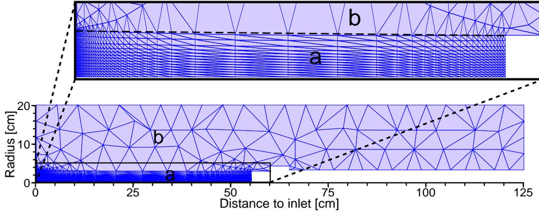
Figure 1: The cylindrically symmetric B2-Eirene grid for Pilot-PSI simulations. Below the complete grid is shown. The triangular grid of Eirene describes the whole computational domain, while the quadrangular grid of B2 is only defined in the region of the plasma, between the inlet at 0 cm and target at 55 cm. The dashed line in the enlarged view indicates the border of area *a*, where both the B2 and Eirene grids are defined, and *b*, which is only defined by Eirene.
