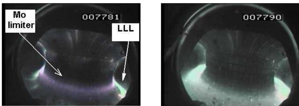
Fig.3 VC pictures of visible light glow w/o high level Li injection (left) and with him (right).
