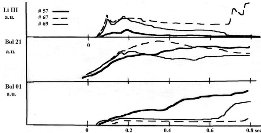
Fig.2. Waveforms of Li-III emission and horizontal B01 and vertical B21 bolometer signals for the shots: #29857 (w/o Li), #29867 (w Li), #29869 (after Li)
