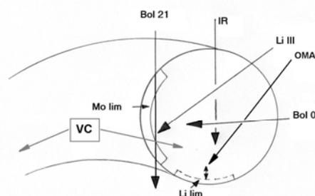
*Fig.1. A simplified scheme of the FTU Li experiment: VC- CCD Camera, Bol 01 and Bol 21 – horizontal and vertical channels of the bolometer array, IR –infrared sensor for measurements of Li limiter surface temperature, OMA – optical multi-channel analyzer*
