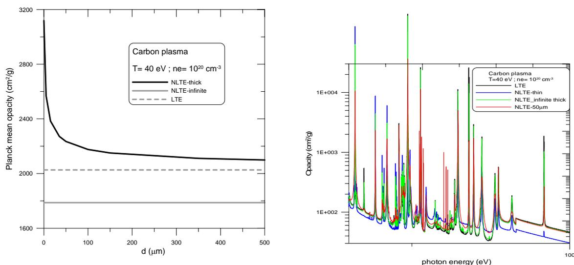
**Figure 2.** Planck mean and spectrally resolved opacities for a carbon plasma.
