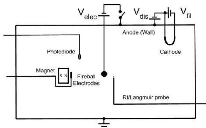
Fig. 1: Schematic of the experimental setup, the Innsbruck DP-machine, where the separating grid was removed in order to create a greater volume of homogeneous plasma. The plasma confinement is strongly improved by a cage of strong permanent magnets on the inner chamber walls.
