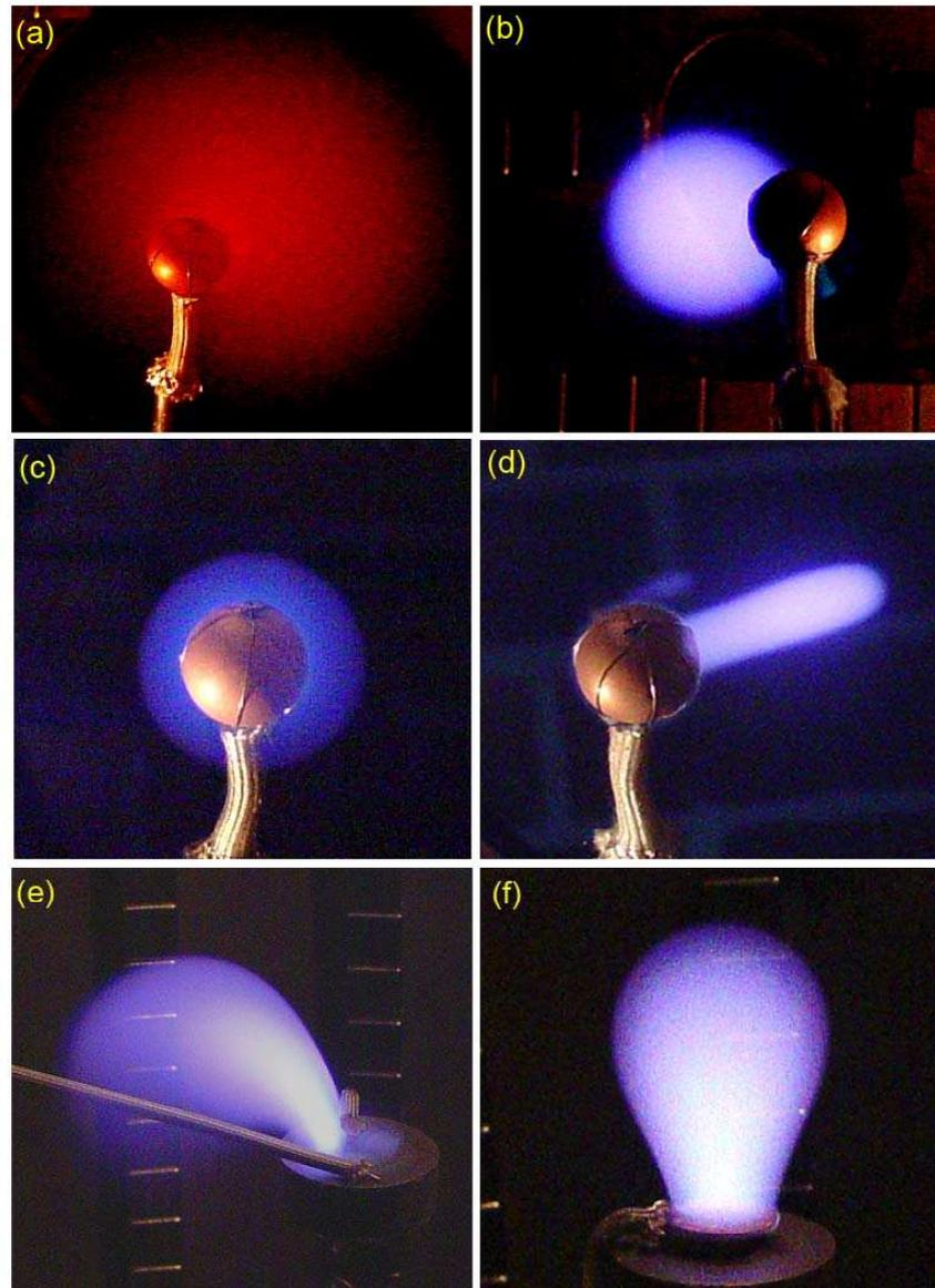
*Fig. 2. Images of different fireball formations: (a) Unstable fireball in neon, which appears diffuse due to fluctuations. (b) Stable spherical fireball on argon whose sharp boundary indicates the presence of a double layer. (c) Luminous sheath at voltages below the threshold for fireball formation. (d) Firerod in an unmagnetized argon plasma. (e) Fireball in hydrogen in a dipole magnetic field off-axis and (f) on axis.*
