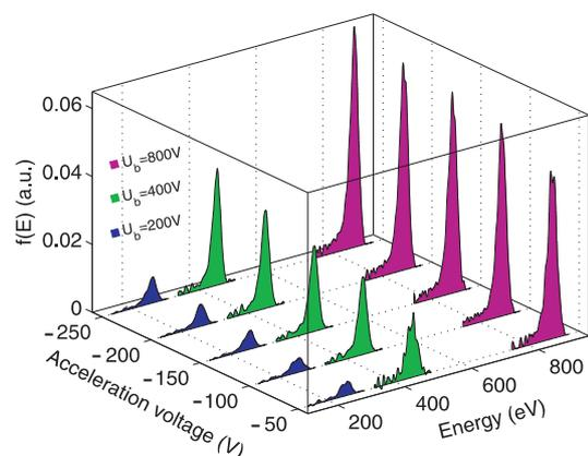
**Figure 6:** IEDF dependence on the accelerator potential. Colors indicate the corresponding anode potential.
