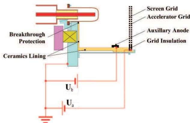
**Figure 2:** Schematic drawing of the IS discharge vessel and electrical circuits [6].
