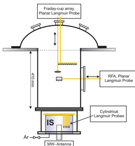
**Figure 1:** Schematic of the experimental set-up (VIBEX).
