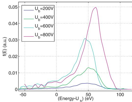
**Figure 4:** IEDF for different beam energies. The x-axis is normalized to the anode potential. Line color denotes the set ion energy as shown by the legend.
