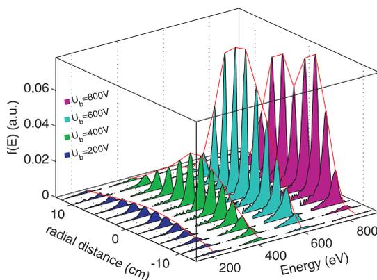
**Figure 5:** Radial IEDF profiles at different beam energies. The external read line is extrapolated from IEDF maximum for every radial position of the analyzer.
