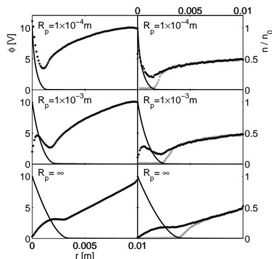
Figure 2: Normalized concentrations of electrons (black) and negative ions (grey) on right y axis and potential distribution on left y axis as functions of the distance from the substrate  $r$ . Cylindrical geometry. Left – relative concentration of negative ions 0%, right – relative concentration of negative ions 50%. Parameter – radius of the probe.
