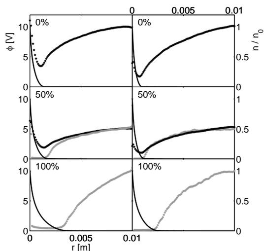
Figure 1: Normalized concentrations of electrons (black) and negative ions (grey) on right y axis and potential distribution on left y axis as functions of the distance from the substrate  $r$ . Cylindrical geometry. Left – pressure 133 Pa, right – pressure 1330 Pa. Parameter – relative concentration of negative ions. Density of undisturbed plasma is  $n_0 = 1 \times 10^{15} \text{ m}^{-3}$  for 133 Pa and  $n_0 = 3.16 \times 10^{15} \text{ m}^{-3}$  for 1330 Pa.
