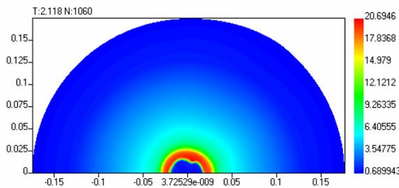
Fig.3. Density ( $\text{g/cm}^3$ ) distribution over the target.
