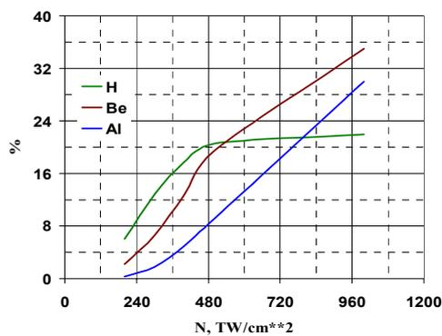
Fig.6. Converter efficiency as a function of ion beam intensity for different materials
