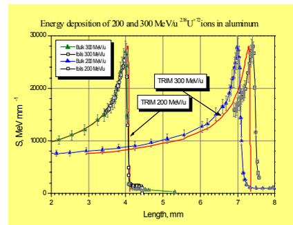
Fig.2. Experimental results of ion beam stopping measurements in condense matter (SIS18 accelerator, VNIIEF, GSI and ITEP groups, “thick target” method [4])
