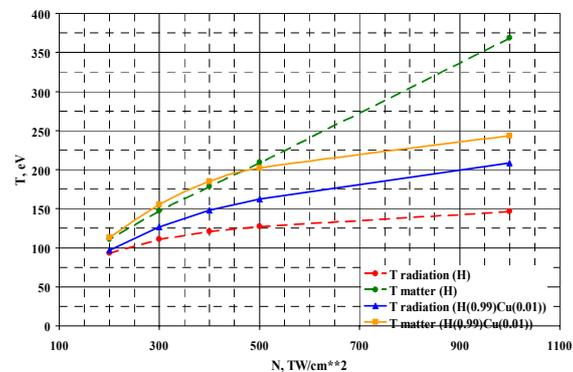
Fig.7. Converter temperature as a function of ion beam intensity for different materials composition
