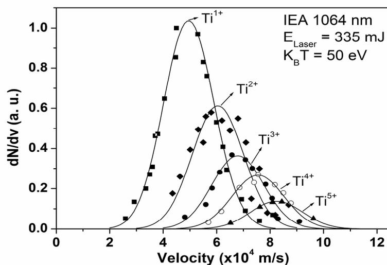
**Fig. 2** : Ion energy distribution as a function of the Ti charge state, giving a fit equivalent temperature of 50 eV.
