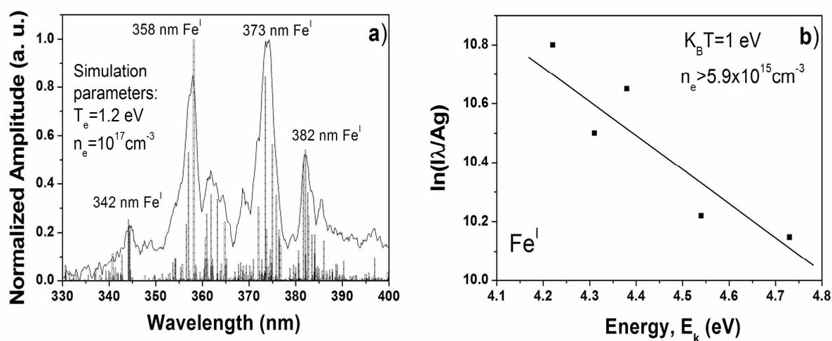
**Fig. 1** : Comparison between the experimental OSS and theoretical spectrum in the region 330-400nm wavelength (a) and Boltzmann plot of the optical spectroscopy analysis giving a coronal plasma temperature of 1 eV from Fe<sup>I</sup> de-excitation lines.
