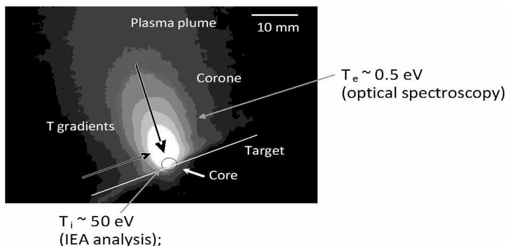
**Fig. 3** : CCD optical image of the Ti plasma plume expanding in vacuum.
